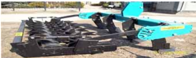
Chisel cultivator type CC
